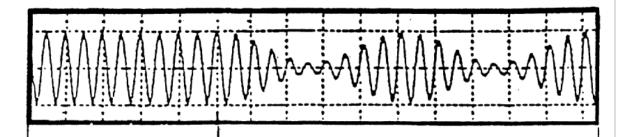
Unmodulated sine wave whose rms value is as defined in Section 6.4.2 of Annex I
