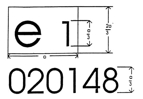
The ESA bearing the above EC type-approval mark is a device which has been approved in Germany (e1) under the base approval number 0148. The first two digits (02) indicate that the device conforms with the requirements of Directive 75/322/EEC, as amended by Directive  $2000/2/\text{EC} \otimes 1$ .
