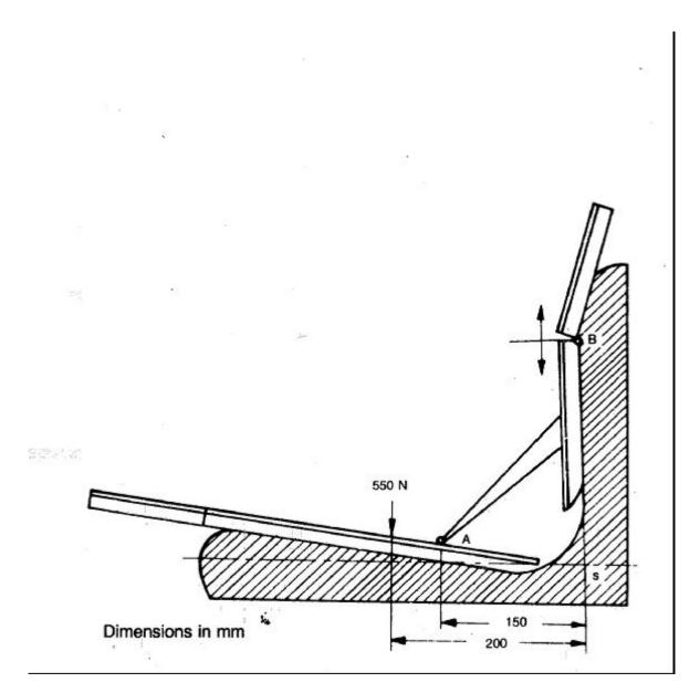
$Figure \ 8$  Method of determining seat reference point
