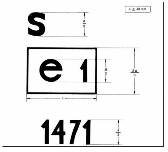
The protection structure bearing the EC component type-approval mark shown above is a  $\boxtimes$  protection  $\boxtimes$  structure for which EC component type-approval was granted in Germany (e 1) under the number 1471.
