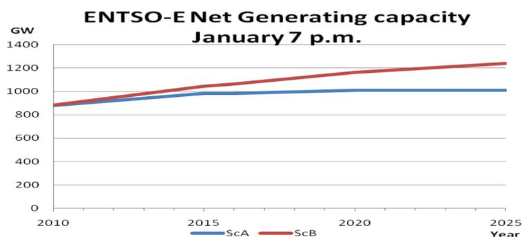
Generation adequacy can be assessed by comparing the difference between demand and reliably available capacity, which is referred to as Remaining Capacity. The table below shows that Remaining Capacity is positive, however, given a low level of new generation development under Scenario A, the level declines sharply after 2015.
